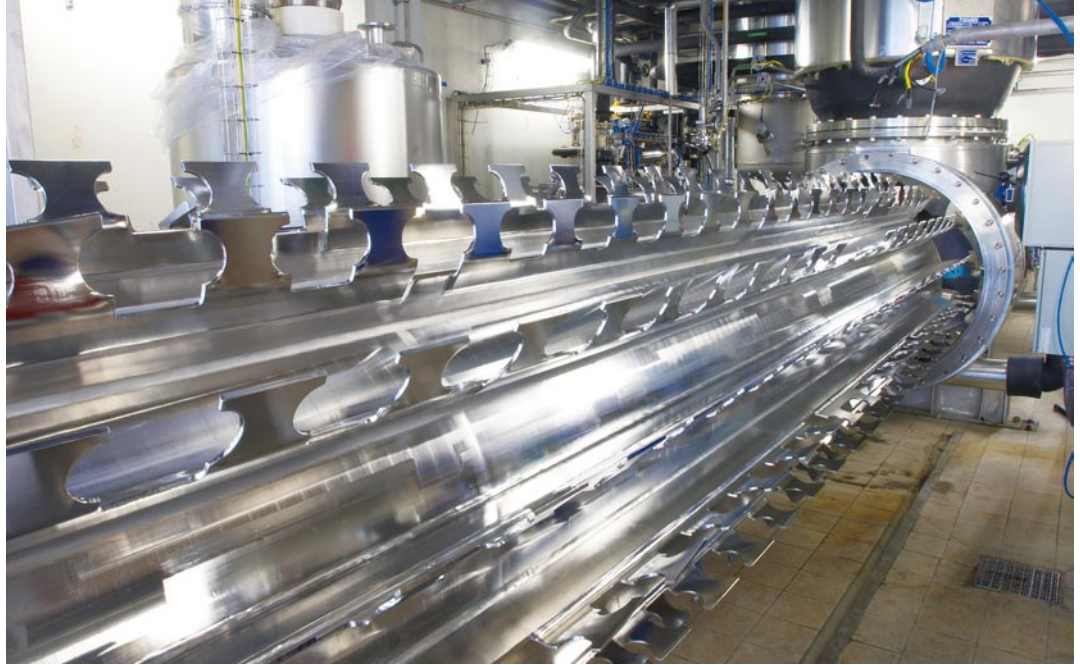
Thin Film Dryer Type Contivac NDP
